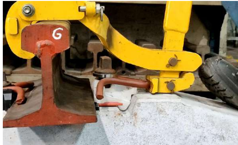
SD Preassembled up to 40 N.m
