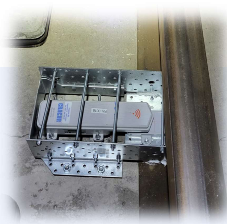
Figure 17 - Sensor 18 with the metal cage to protect against accidental blows and impacts from trains (Photo: Trigonet, 17.06.2024)
