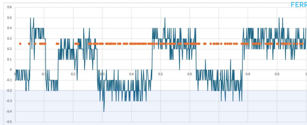
Figure 30 - Graph of the displacements detected by sensor C-13, in direction Y, on 24 hours of the day 24.7.2024 (CIPM2020)
